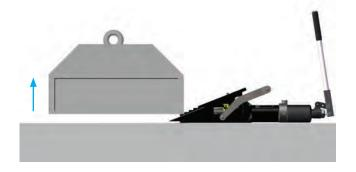
The load is secured using the safety block
