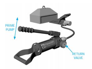
5. Once the item has been lifted to the desired height, or to the maximum height on the step used, the safety block should be inserted into the gap. Secure the load by releasing the pressure onto the block.
