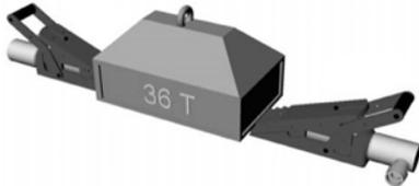
Using four VLW18TE/TI wedges will allow a lift of 72 Tons
