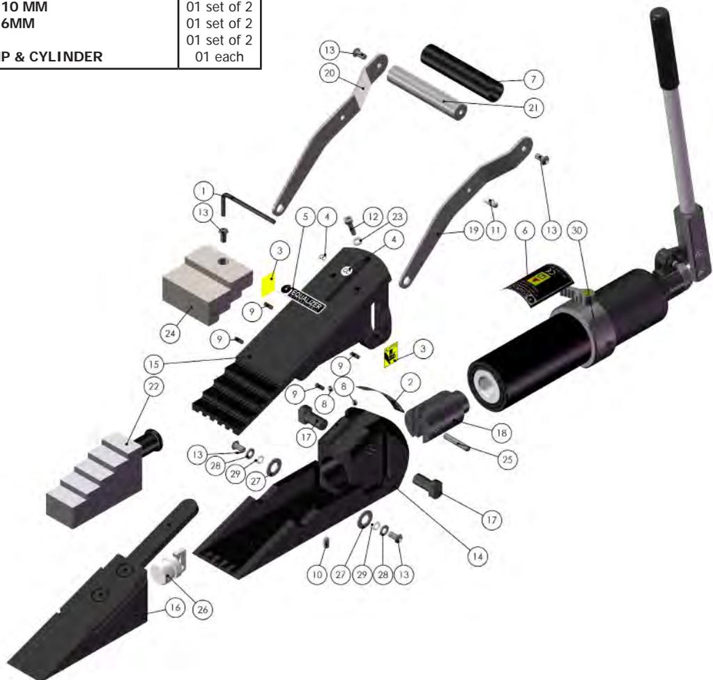
**INTEGRAL HYDRAULIC PUMP/CYLINDER serial no: 11187 onwards**
