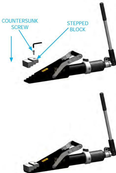
Insert the tool under the item to be lifted. Ensure there is a minimum hold of 15 mm (0.59") and that the full width of the block is used
