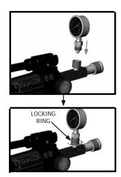
2. Ensure the hydraulic system you wish to pressurise has been bled and is free from air and leaks.
