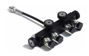
Each tool can be independently isolated by closing the corresponding valve. It is not recommended to isolate or engage alignment tools while under load as an overload might occur. See the document 'Use of Equalizer International tools with a Hydraulic Manifold' for further guidance.
