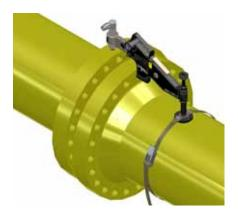
Connect the hydraulic pump to the hydraulic hose, and the hose to the hydraulic adjusting cylinder.
