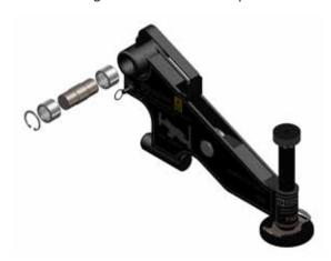
Remove the spirol retaining clips from the lower shaft and slide the shaft out from the main body.
