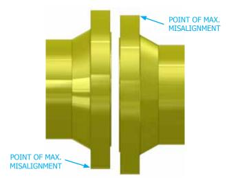
Guide the lift hook into the bolt hole at the point of maximum misalignment.
