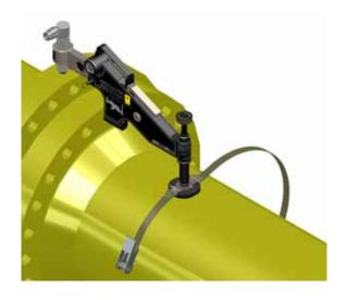
Feed the open end of the strap through the ratchet mechanism as shown. Tighten the strap using the ratchet mechanism.
