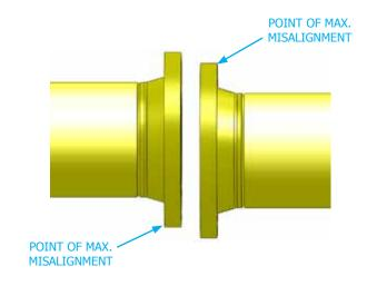
Guide the lift hook into the bolt-hole at the maximum point of misalignment.
