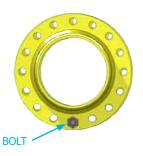
**3.** Repeat steps 1 and 2 at other points around the flange until all of the remaining bolt-holes are parallel and the rest of the bolts can be insterted.
