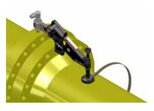
Now place the hook of the ratchet mechanism through the base on the opposite side as shown.
