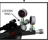
2. Ensure the hydraulic systems you wish to pressurise have been bled and are free from air and leaks. Connect the pump into the systems using the screw connectors supplied with the pump, push the male and female connectors together fully and rotate the locking rings clockwise until fully tight.
